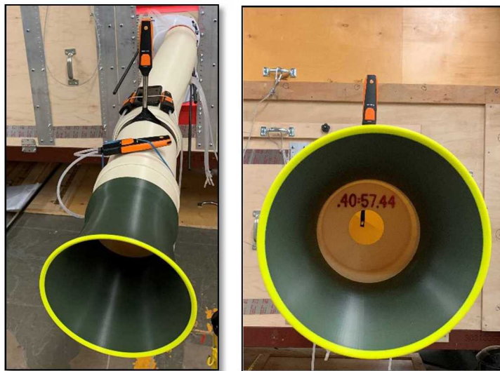
Fig. 4 Duct inlet outside the wind tunnel with choke section and close-up of choke and hot wire anemometer.
