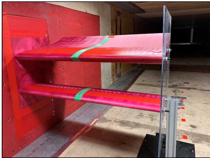
Fig. 2 A 0.5 m chord AeroMINE pair mounted in the wind tunnel. The green ribs contain static pressure taps along the low-pressure side of the foils.
