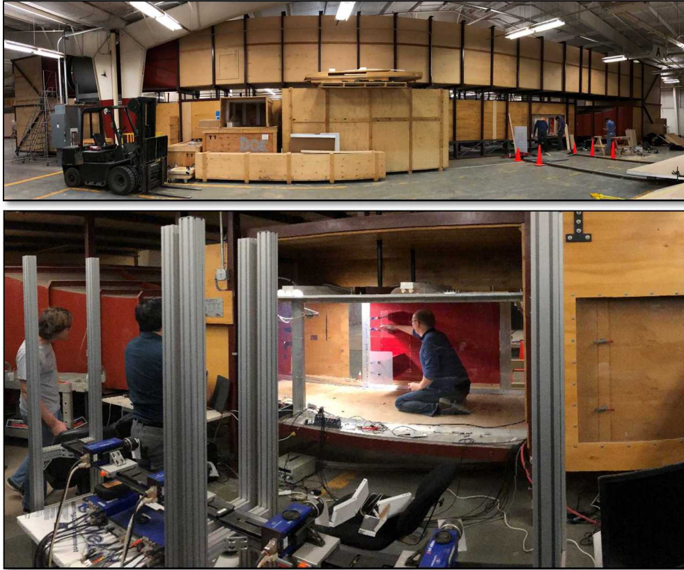
Fig. 3 Wide-angle photos of both sides of the National Wind Institute wind tunnel at Texas Tech University, including the PIV camera array on the transparent side, looking into a smaller array of 2 AeroMINEs.
